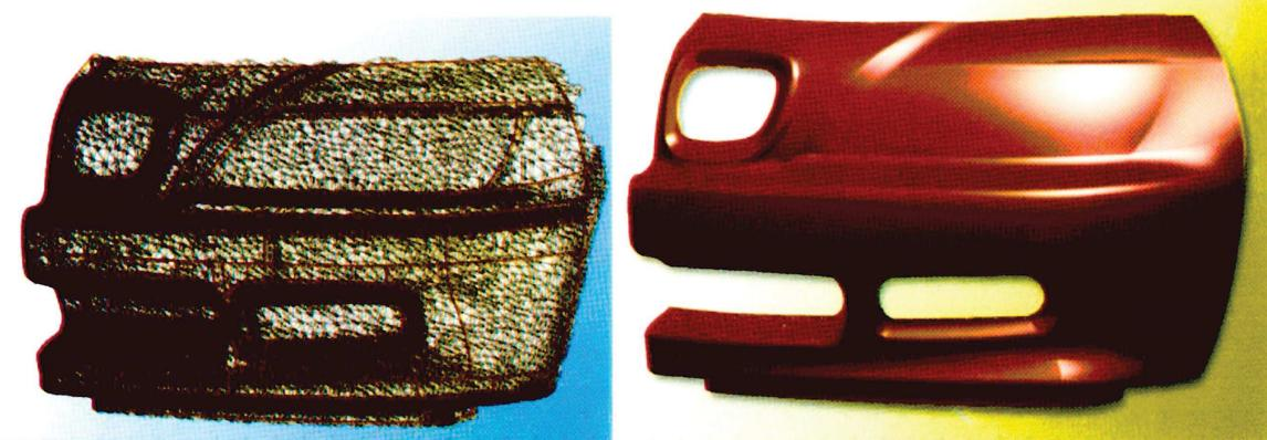
*Figure 6 „Cloud of points“ with s triangular net and smoothed surface model in ICEM Surf [7]
