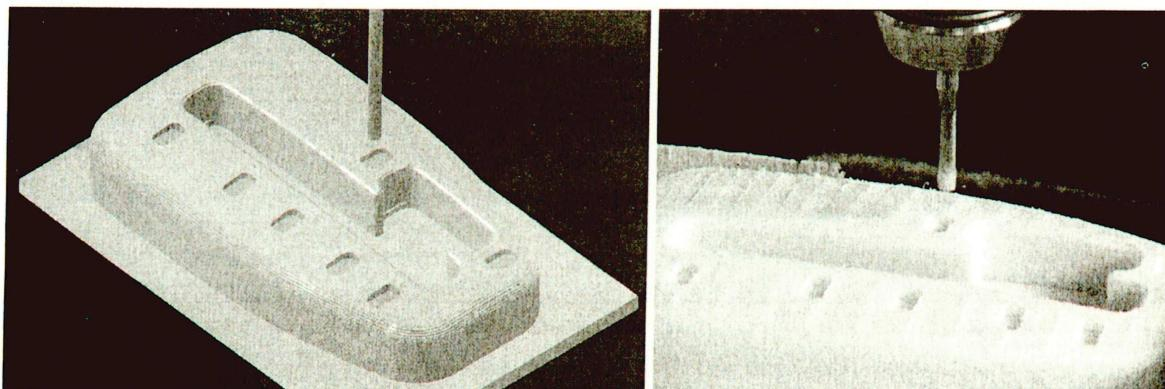
*Figure 7 Simulation of tool path and a model production [3]
