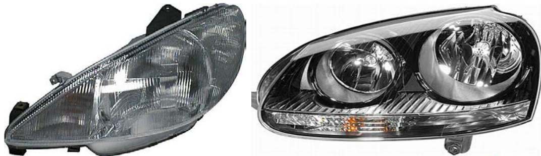
Fig.7 The difference between the reflector optics on the cover glass with clear cover glass optics with the dish
