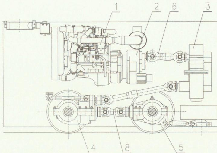
Figure 9 Diagram of drive transmission in Lds-100 locomotives
