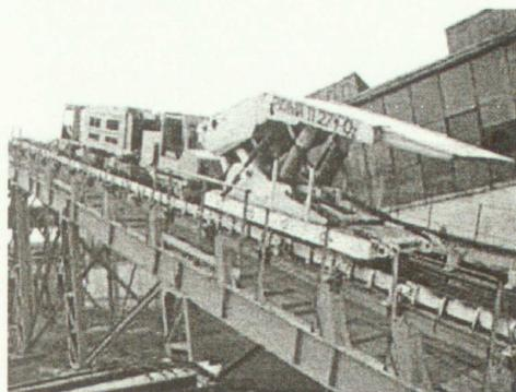
Actuating driving system consists of four repeatable driving modules-cars (Fig. 3), where the cabins and diesel-and-hydraulic units are installed. Articulated joints couple the modules with each other, and each joint is secured by two safety ropes. Each module has a driving system consisting of two hydraulic engines, which drive the frictional wheels and rack wheels as well as a shoe brake system, which
