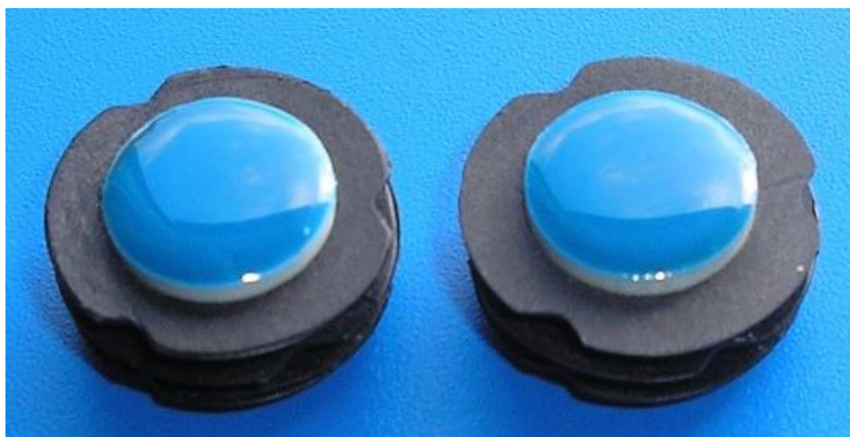
Figure 13 Tags applied in Chemosvit, Inc. for steel press rollers
