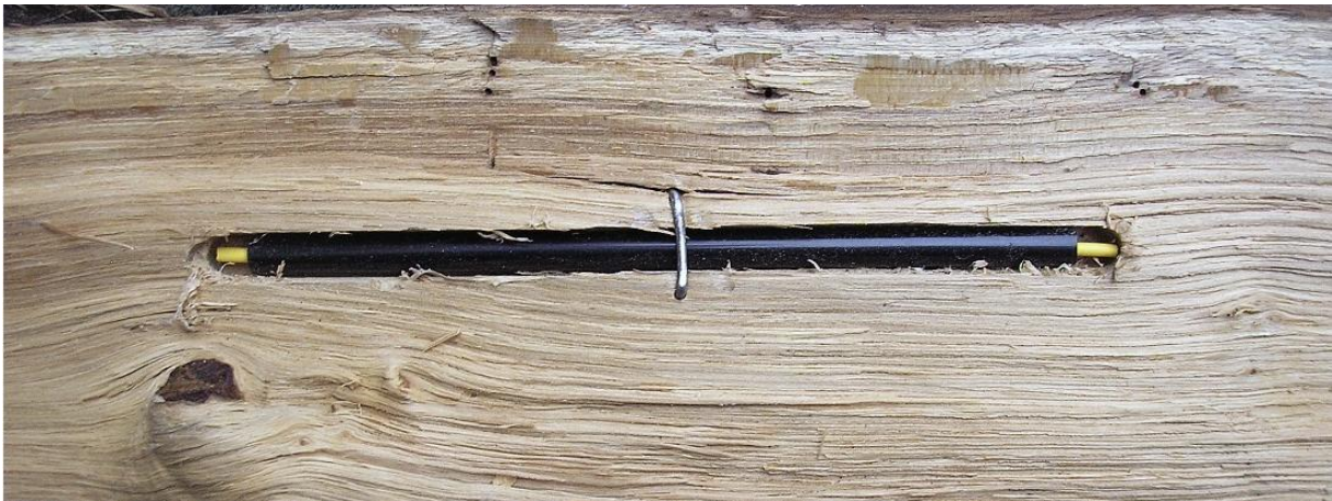
Figure 12 Tag that allows flush mounting to wood, designed for recording the mining in forests
