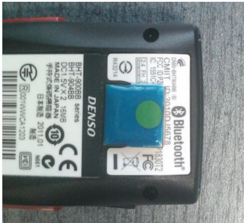
Figure 8 Evidence of measuring instruments (tags on metal 15x15x1,5 mm)
