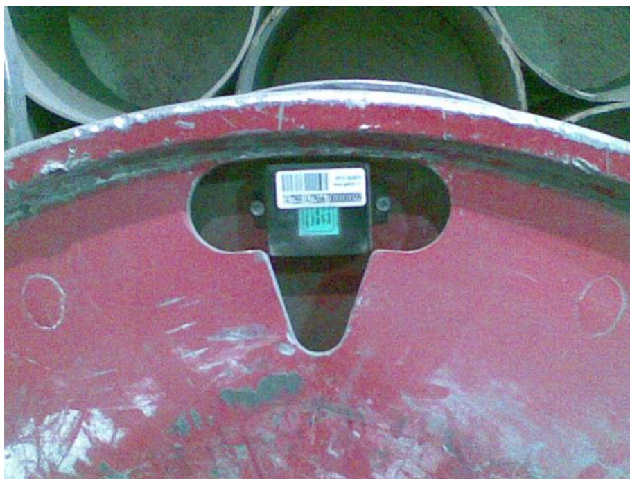
Figure 9 Placing tags on metal drums for a record of production of metal wires
