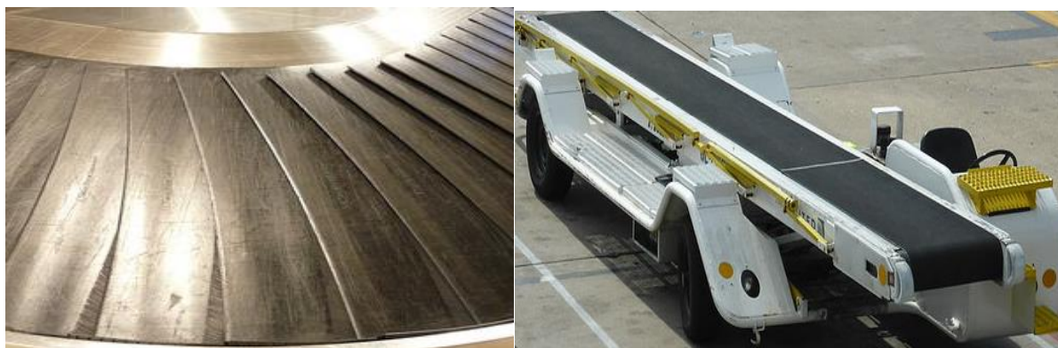
Fig. 1 Belt luggage conveyors in air transport
