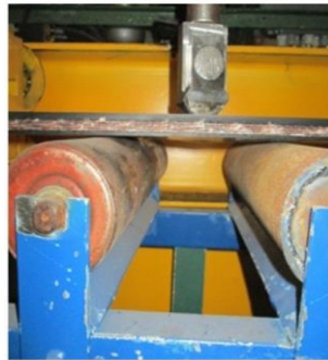
Fig.1 Tensioned conveyor belt with a support system and a pyramid impactor
