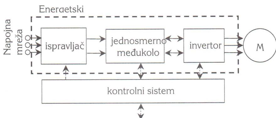
Figure 1 Simplified diagram of frequency converter
