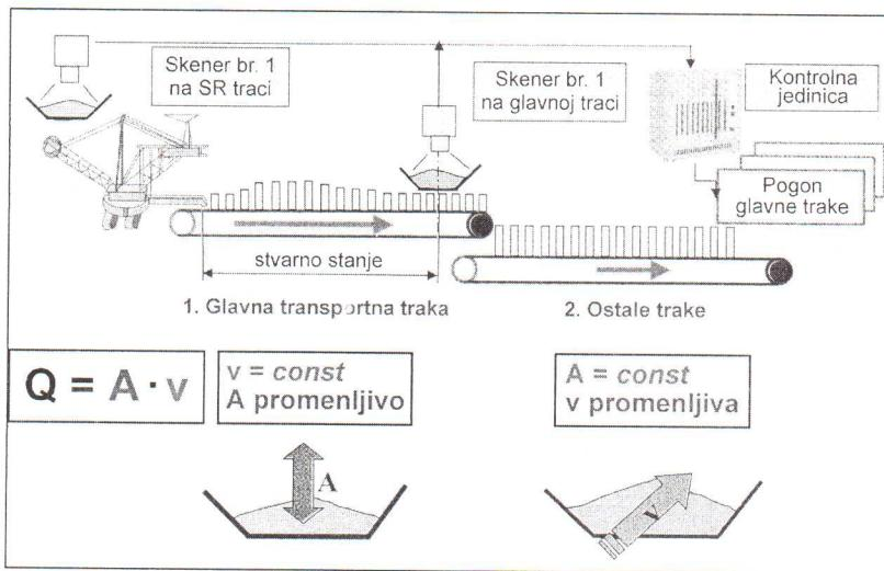
Figure 3 Conceptual layout demonstrating loading control and frequency regulation of belt conveyors
