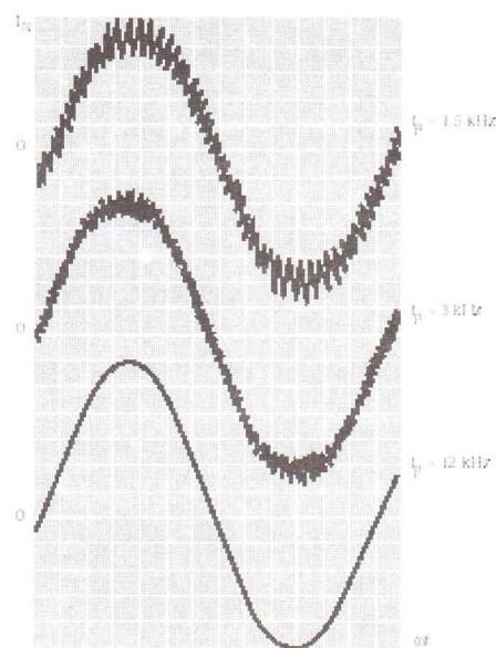
Figure 2 Motor current at different inverter breaker frequencies
