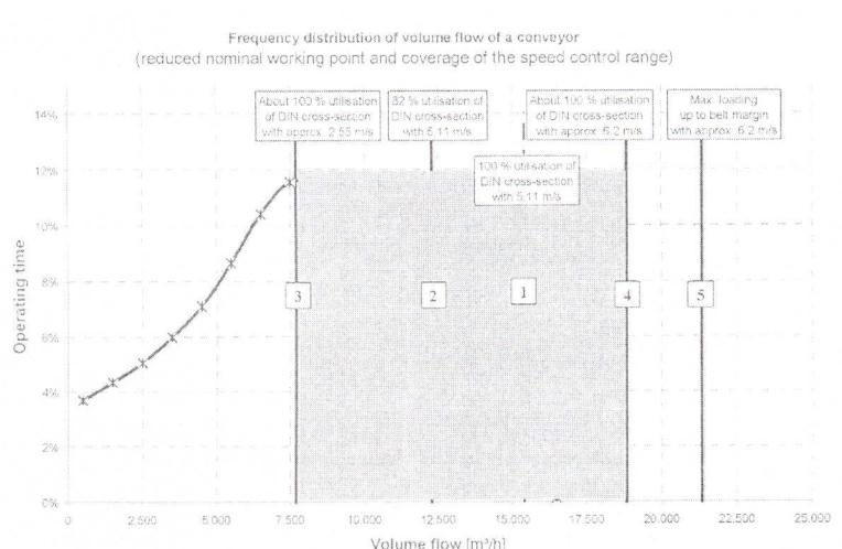
Figure 6 Flow rate regulation procedure
