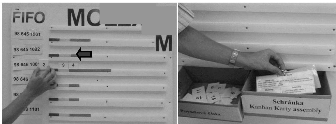
Obr. 11 Zmena stavu FIFO tabule po vyskladnení dielov k projektu Fig. 11 Change in FIFO board after removal of parts of the project
