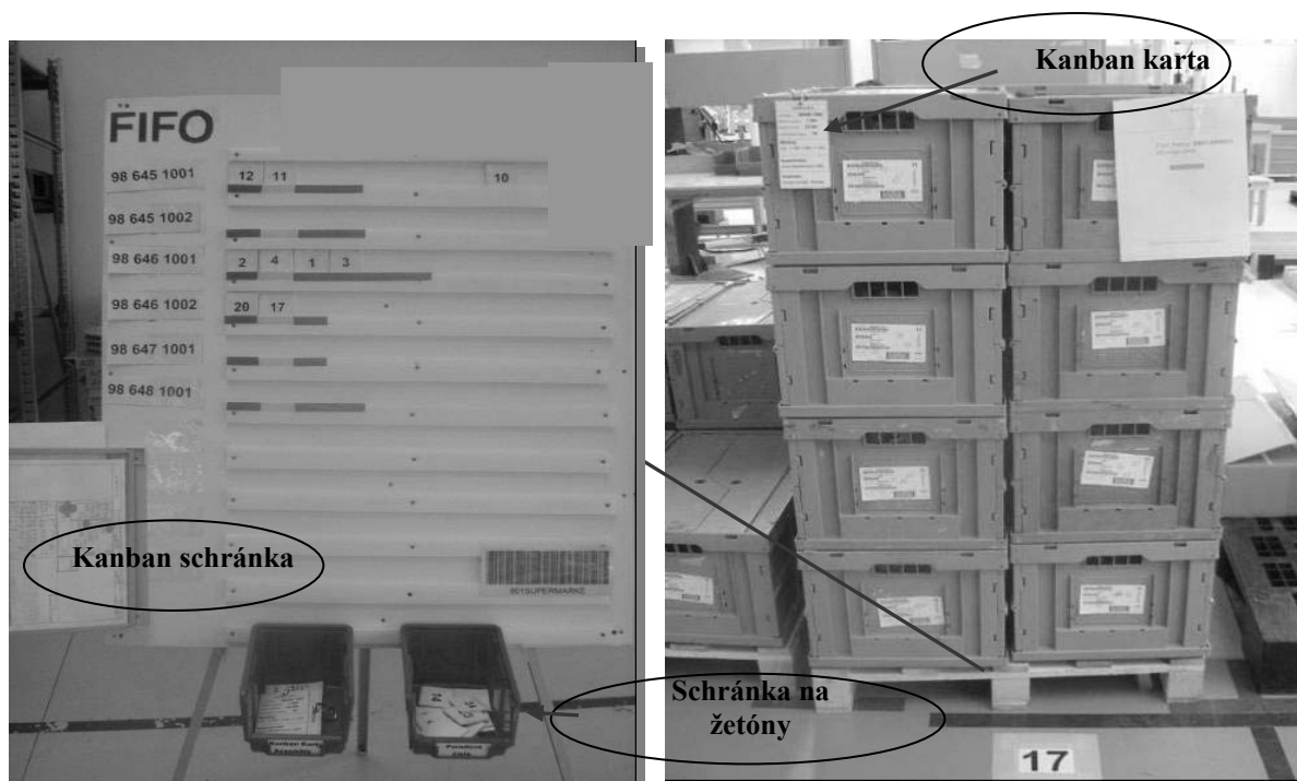
Obr. 8 Prehľad FIFO tabule a uskladnenie paliet v supermarkete Fig. 8 Overview of FIFO board and storage pallets at the supermarket
