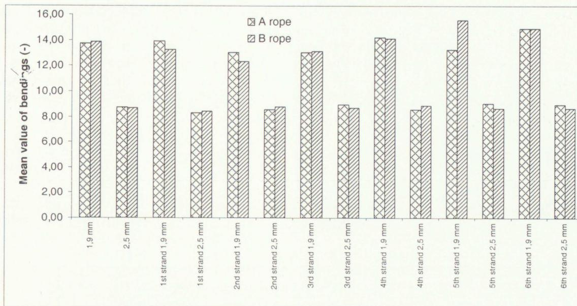
Figure 3 Mean values of wires bendings of complete ropes and particular strands by wires diameters
