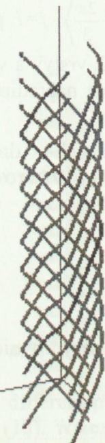
**Fig. 7 Axes of wires of the 1<sup>st</sup> layer**
