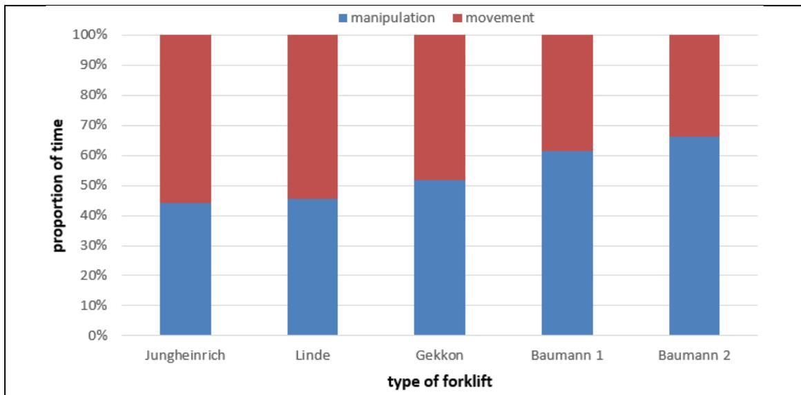
*Fig.2 The proportion of time for the movement and manipulation operations (loading and unloading)*
