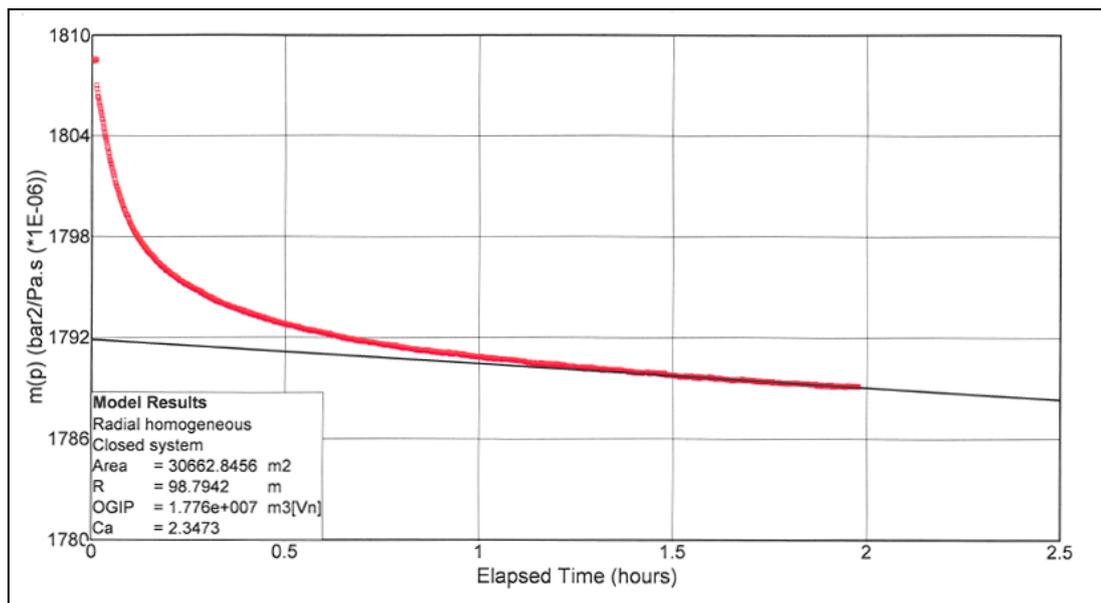
**Fig. 5** Cartesian plot for a closed system.
