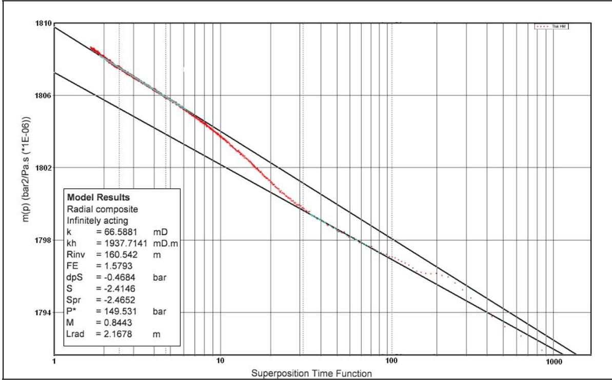
Fig. 2 Radial flow plot for a radial composite flow.
