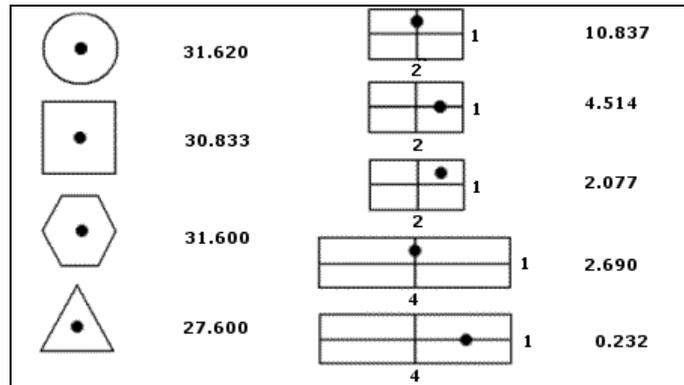
**Fig. 4** Constant rate Dietz shape factors [3].
