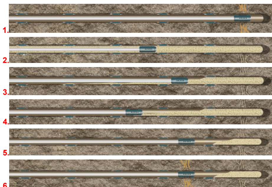
Fig. 5 Jet perforation and stimulation of the zones inside expandable tubulars [12].
