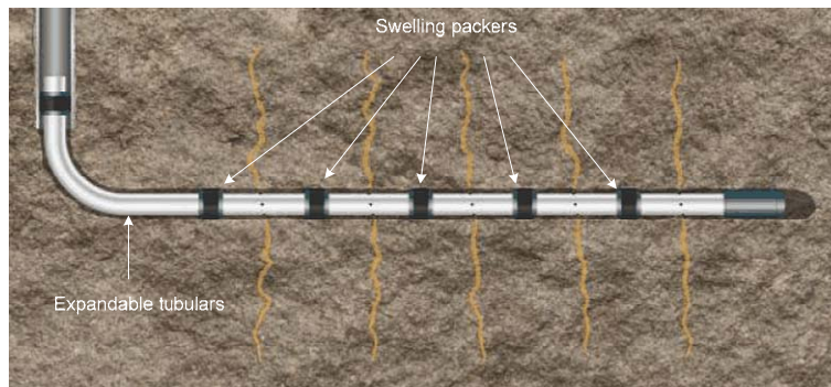
Fig. 6 Expandable tubulars in tandem with swelling packers providing for effective pay zone stimulation [12].
