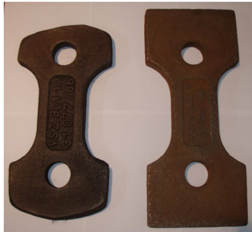
Fig. 4 Deteriorated and new coal crusher hammer
