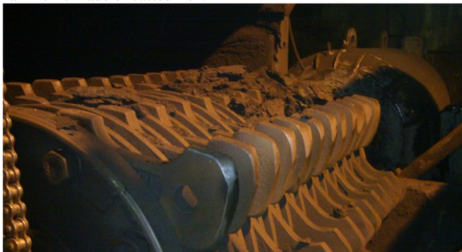
Fig. 3 Coal crusher – view of the hammers
