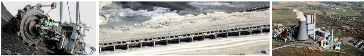
Fig. 3 Example of a connection supplier and customer by belt conveyors
